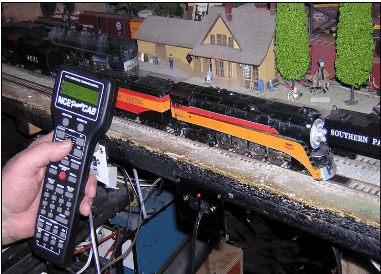
Testing the Power Cab to see how it works when used on the program track. It read back the Tsunami sound decoder CVs with no problems. Another new feature was the playable whistle. I set up the playable whistle and used it on the Daylight. That also worked OK.
